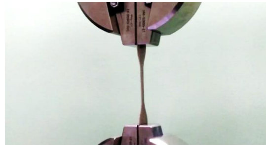
Figure 6. NFRP sheet testing
