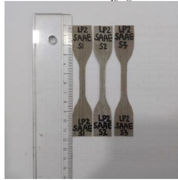
Figure 5. Detail specimen of NFRP sheet
