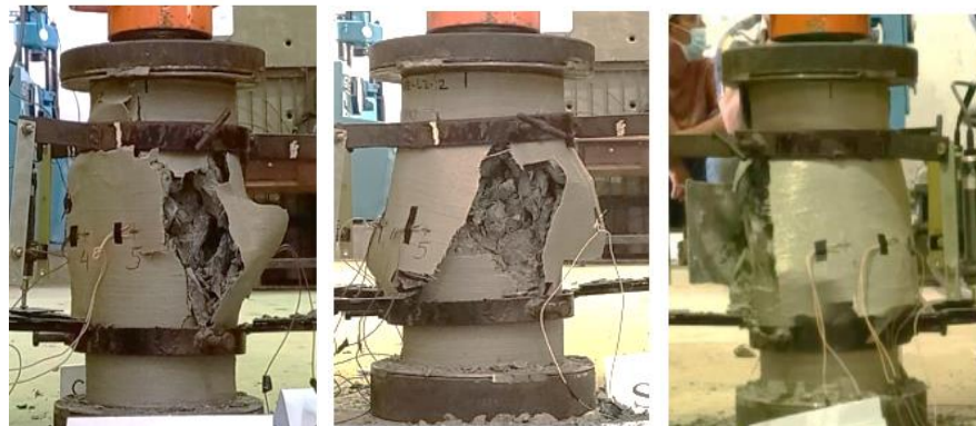
Figure 9. The failure mode of NFRP-confined concrete
