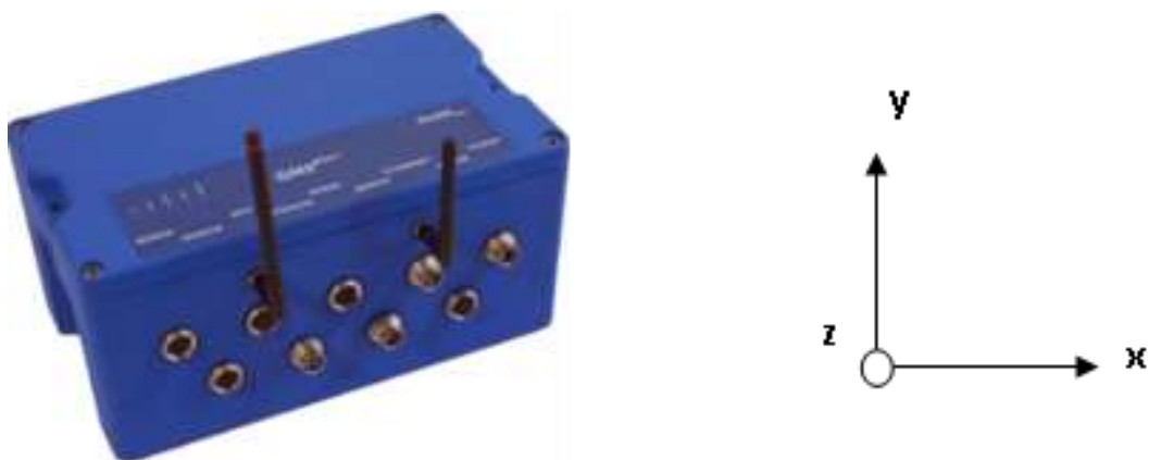
Figure 4. GeoSig accelerometer and its direction
