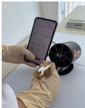
Figure 3. The composite tube was heated in the composite heater for 15 min at 60°C.
