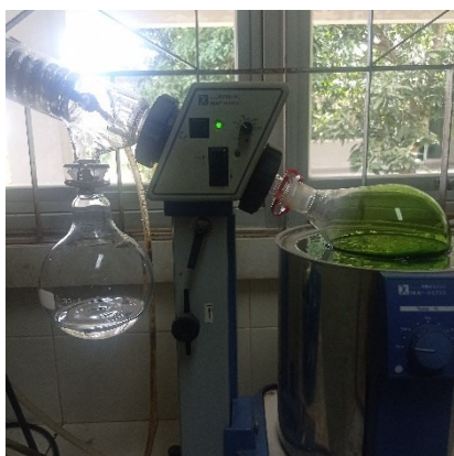
Figure 2. Evaporated filtrate of Sungkai leaves ( Peronema canescens Jack.) using a rotary evaporator
