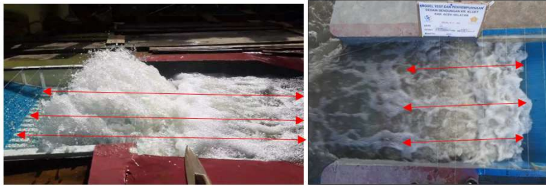
Figure 15. Visualization of S_0 (left) and S_1 model (right) hydraulic jump on the Q100 discharge
