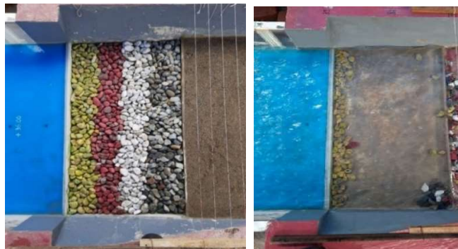
Figure 21. The rip-rap of the S_0 model condition before and after flowing 100 years discharge (Q100)
