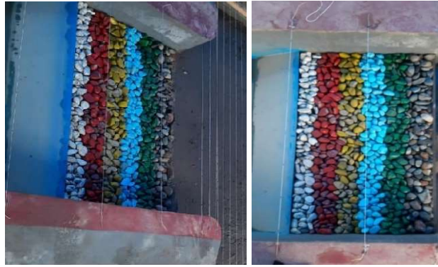
Figure 21. The rip-rap of the S_1 model condition before and after flowing 100 years discharge (Q100)
