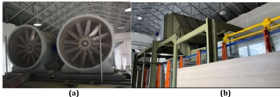
Figure 4. The coaxial fans placed on the top of the flume (a) and the air flow straightener (b).
