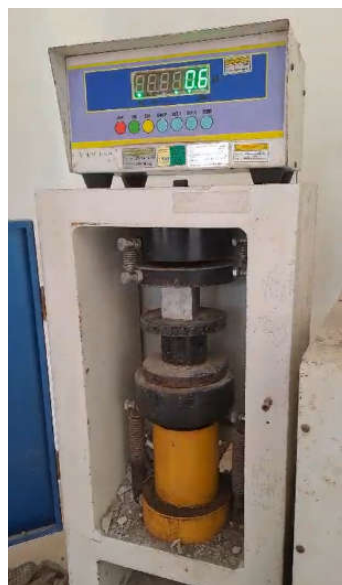
Figure 3. MBT testing machine capacity of 500 kN
