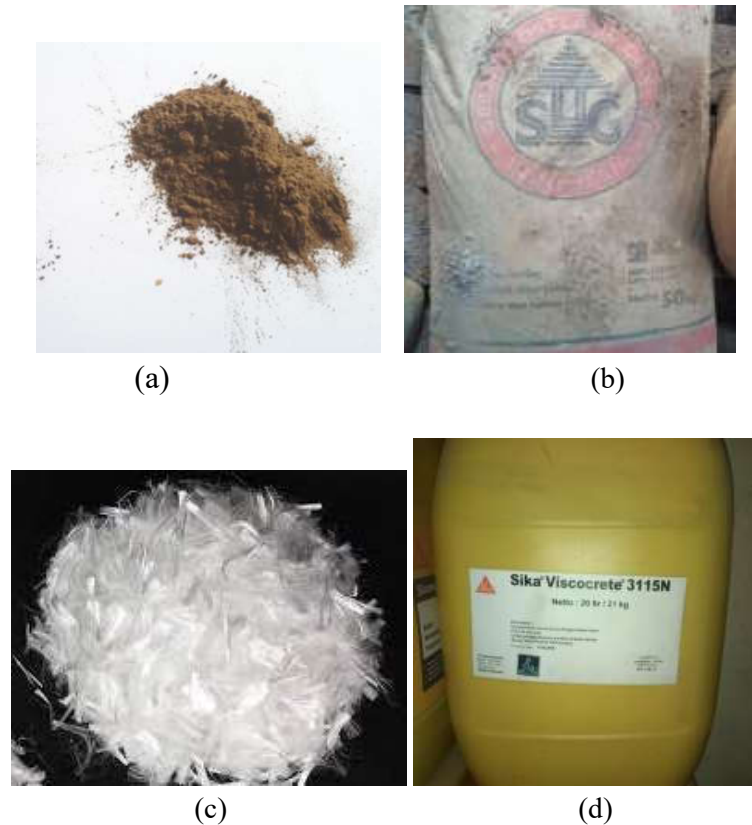
Figure 1. Research materials (a) fly ash, (b) cement, (c) polypropylene fiber, and (d) superplasticizer
