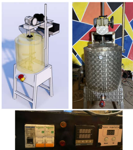
Figure 1. Machine Design (a) 3D CAD (b) Mixing Machine (c) Machine Control Panel Source : Research Documentation, 2024
