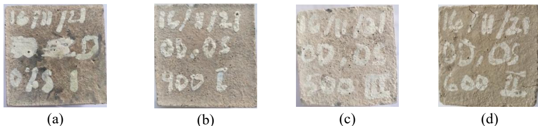
Figure 1. High-strength concrete without diatomaceous earth and with 0% fiber content: (a) at room temperature, (b) after heating at 400°C, (c) after heating at 500°C, (d) after heating at 600°C.
