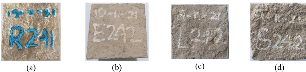
Figure 9. High-strength concrete with 10% diatomaceous earth substitution and 0.6% fiber content: (a) at room temperature, (b) after heating at 400°C, (c) after heating at 500°C, (d) after heating at 600°C.
