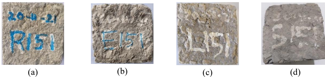
Figure 5. High-strength concrete without diatomaceous earth and with 0,8% fiber content: (a) at room temperature, (b) after heating at 400°C, (c) after heating at 500°C, (d) after heating at 600°C.
