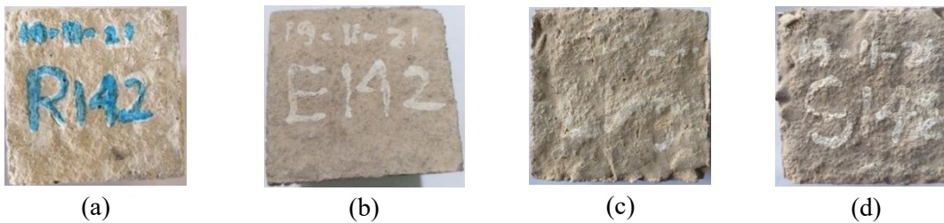
Figure 4. High-strength concrete without diatomaceous earth and with 0,6% fiber content: (a) at room temperature, (b) after heating at 400°C, (c) after heating at 500°C, (d) after heating at 600°C.
