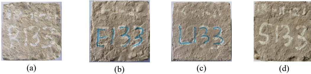
Figure 3. High-strength concrete without diatomaceous earth and with 0,4% fiber content: (a) at room temperature, (b) after heating at 400°C, (c) after heating at 500°C, (d) after heating at 600°C.
