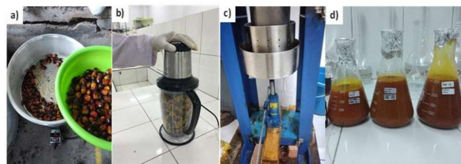
Figure 1. a) Oil palm loose fruits (LF) and steam pans, b) Chopper machine, c) Mechanical press, d) Crude palm oil.
