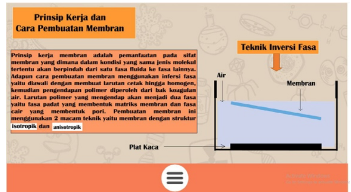
Figure 6. Fundamental theory of inversion phase for membrane formation
