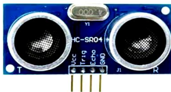
Gambar 5. Sensor ultrasonik HC-SR04
