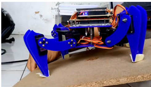
Gambar 10. Hasil mekanik robot quadruped
