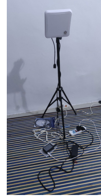
Figure 2. Design of the RFID reader-based item identification device
