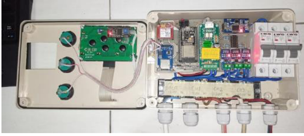
Figure 1. Inside part of data acquisition module
