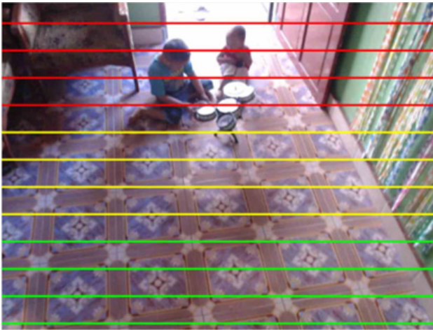
Figure 7. The device detected the children playing in the danger zone
