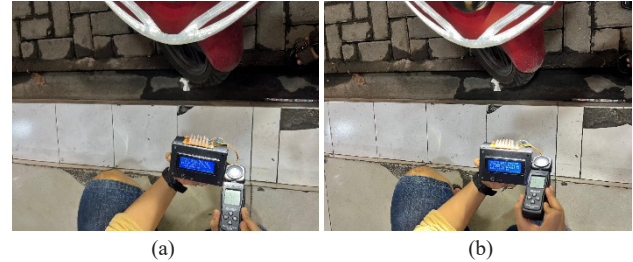
Figure 9. Testing the photodiode sensor array in 4 m × 3 m × 3 m room with: (a) normal mode and (b) sensitive mode
