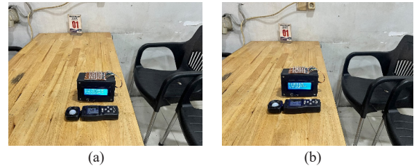
Figure 8. Testing the photodiode sensor array with 10W LED at a distance of 2 m in (a) normal mode and (b) sensitive mode
