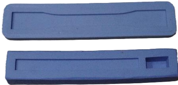
Figure 4 . Mold ASTM D638-I Tensile Test, ASTM D790 Bending Test and ASTM D695 Compression Test.
