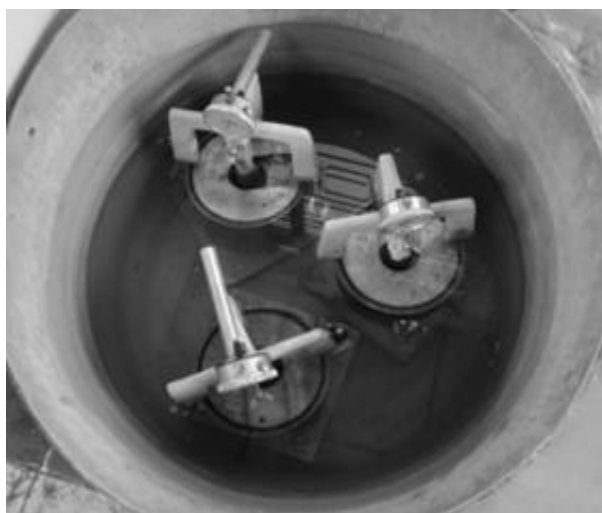
Figure 5. Soaked condition the samples
