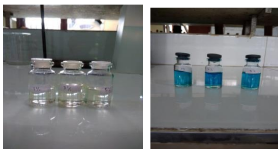
Figure 1. Result of examination of nanoemulsion type in each sample. (A) before dripping with methylene blue, (B) after dripping with methylene blue.
