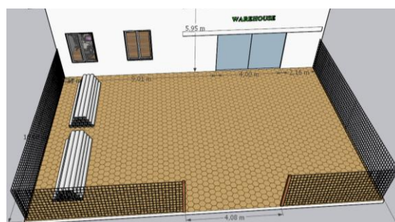
Figure 10. Paving blocks made from plastic waste
