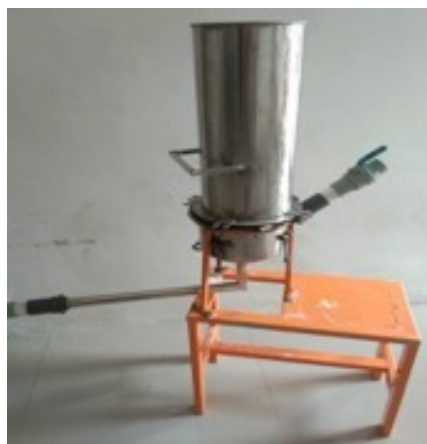
Figure 2. A set of equipment for molding pulp into sheets
